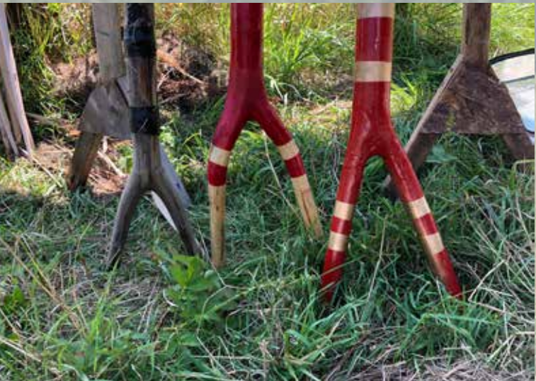
A wooden fork or aluminum “duck bill” is attached at one end of a push pole. Care must be taken to keep all edges smooth on forked ends of push poles to avoid snagging or uprooting plants.
